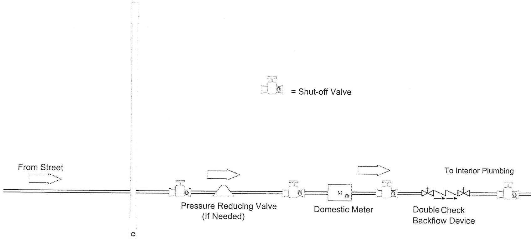
1. All Backflow devices to be installed according to manufacturer's specifications.
