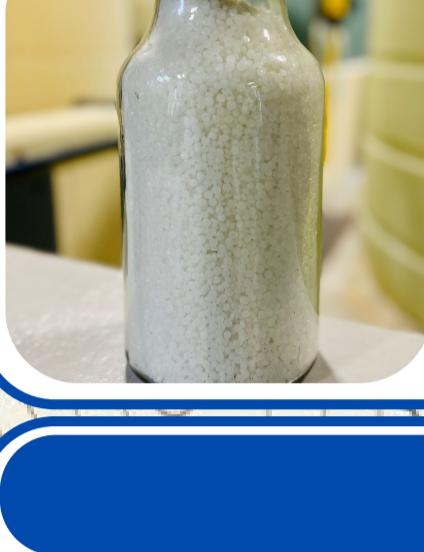
Alum is used in water treatment plants as a coagulant in a critical step to clarify water by causing suspended particles to clump together. When added to water, alum forms flocs that trap impurities, the floc sticks to beads similar to the ones in the photo on the left.
