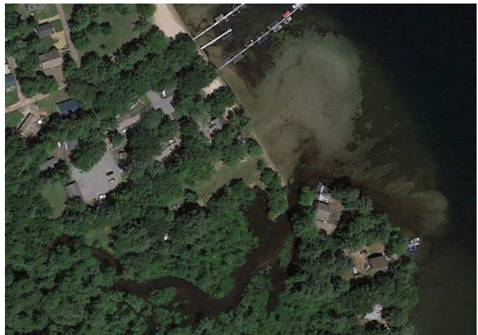
Aerial view of a 300-ft radius sediment delta at the outlet of Black Brook as it enters Lake Winnisquam.
