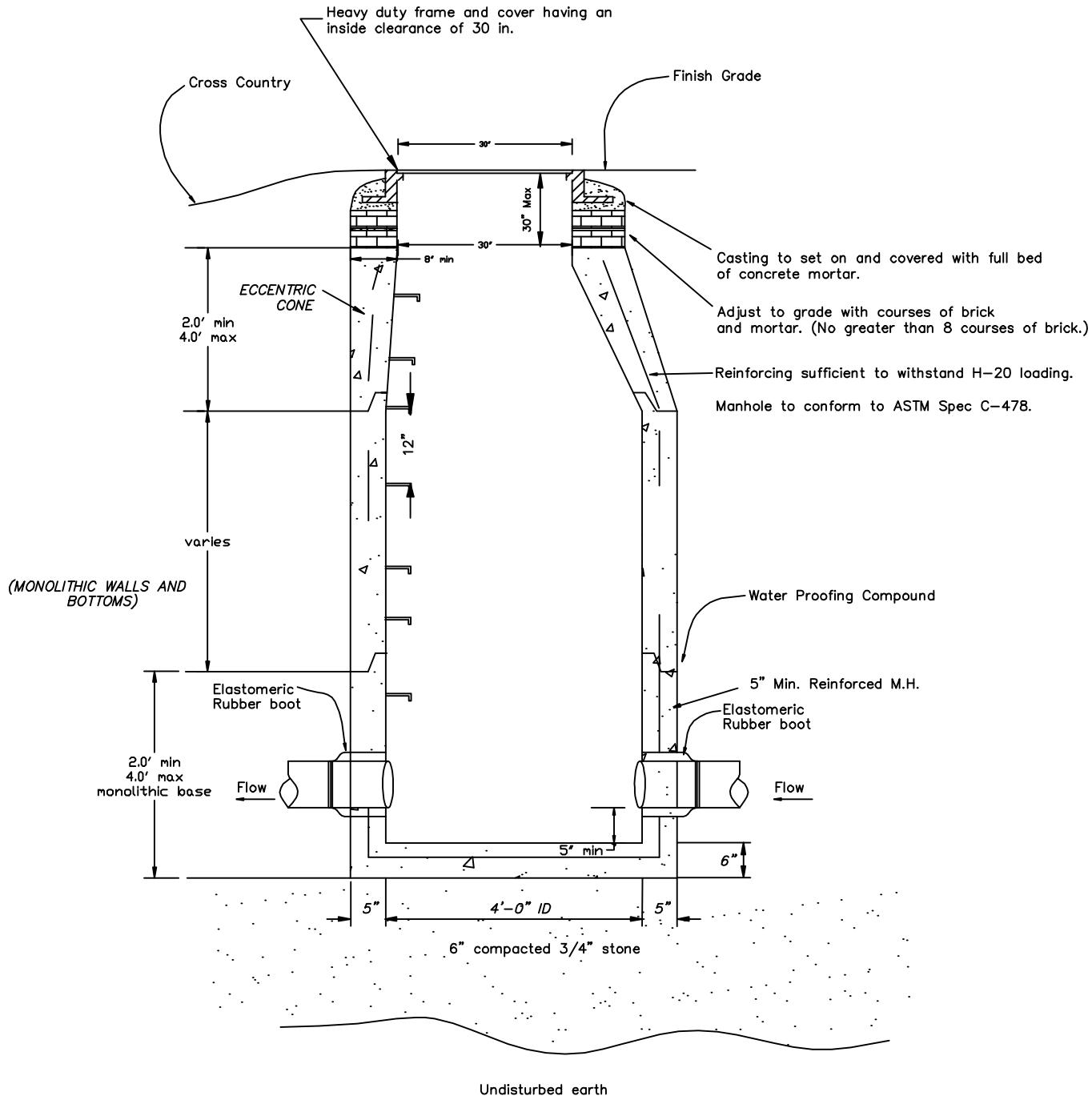
Manhole to conform to ASTM Spec C-478.
