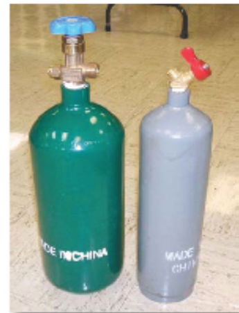
These unauthorized, imported cylinders are sold as part of a consumer welding kit.
